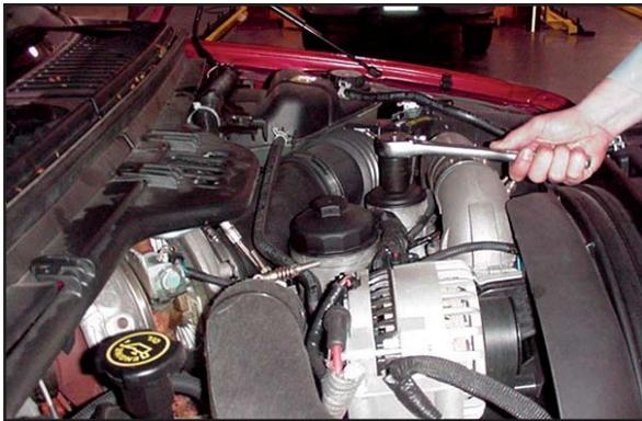
2. Remove fuel filter and O-ring.
