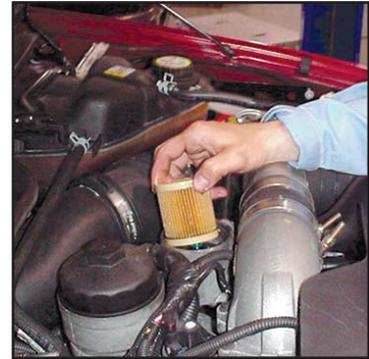
5. Re-attach fuel end cap with new O-ring (provided) back onto the filter housing. Torque end cap to 14 Nm using a 24mm socket or 1/2 inch square drive.
